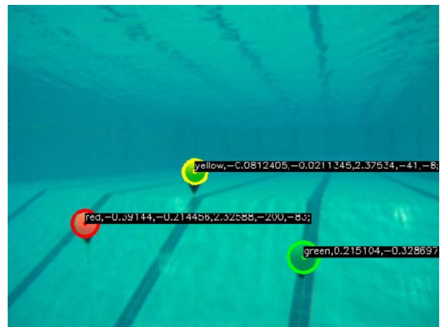
Figure 11 - Debug of the buoy filter chain
